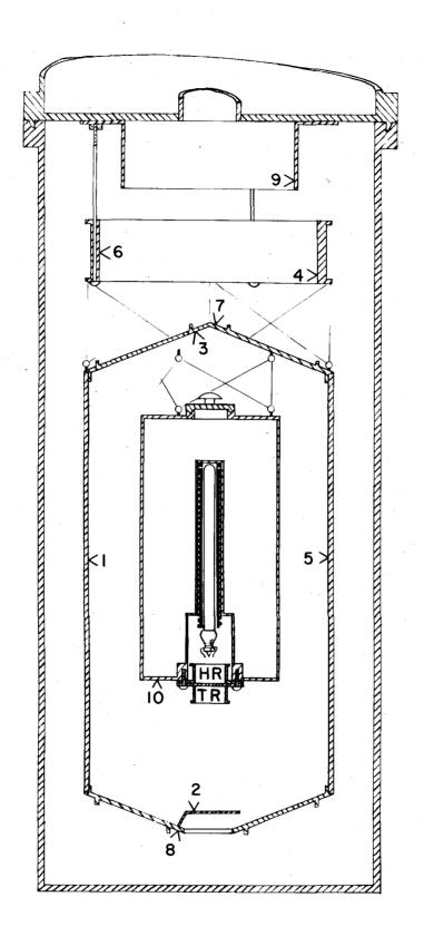
gas port, consisting of a thin walled .066 inch 0.D. copper tube with a top of the can was attached with low-melting indium solder. An exchange flange, was soldered to the top of the can with Sn-Pb solder. The bottom of the can was attached with 50-50 Sn-Pb solder and
